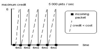
This graphic shows that every 4ms we get 6 credits and we then allow 1 packet to pass which cost 6 credits. We then must wait 4ms before allowing a packet to pass through.
